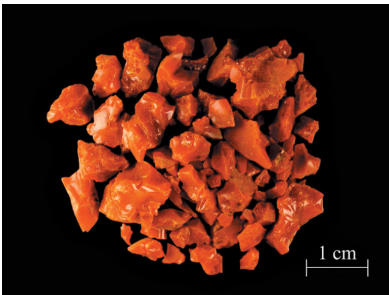
Figure 12. Photomicrograph of Garcinia hanburyi (gamboge) resinous pieces from the Harvard Museum of Natural History and photomicrograph of paper dyed with gamboge.
